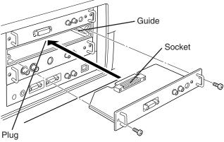
Figure shows HDB 15-PIN terminal (Optional parts).
