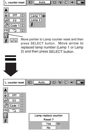
Message "Lamp replace counter Reset?" is displayed. Move pointer to [Yes] and then press SELECT button.
